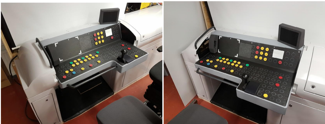
Images of the 1:1 scale mock-up, built into the workshop of LINK Design
