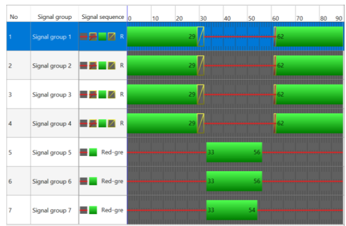
Figure 16. Pedestrian Crossing signal plan
